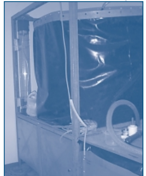
The beneficial microbes housed in this biofilter degrade and oxidize the septic tank effluents.
